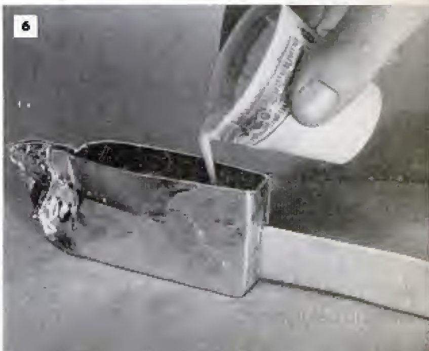
A second aluminum-foil trough is made, this time to enclose the entire knife handle. Holes and joints of trough must be sealed carefully and plastic poured in slowly, as shown below
